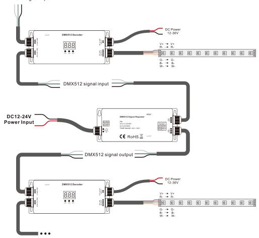
Note: Each amplifier can repeat signal for max. 12pcs DMX512 decoders in parallel within 100m range. More amplifiers are required if there are more than 12pcs decoders and the distance is further than 100m.
